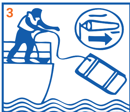
Throw entire life raft overboard in the direction of the wind
