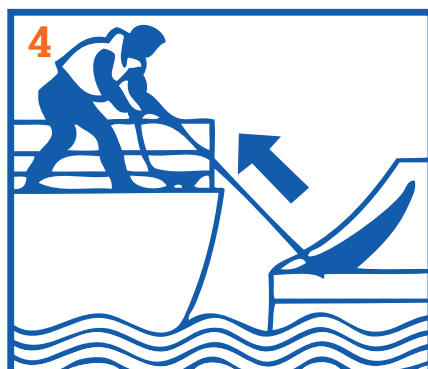
Pull on the painter line to activate inflation mechanism
