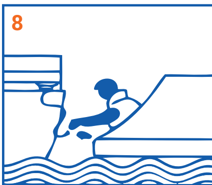
Undo or cut painter line with safety knife located near life raft's entrance
