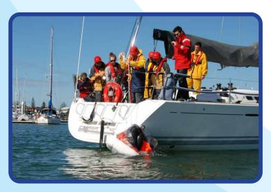
3. Life raft will begin inflation and break its canister's lashing system. A valise packed life raft will break through its polyurethane outer case.
