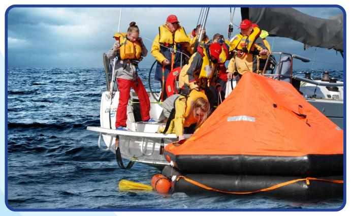
Inflatable life rafts are universally recognised as providing the most efficient method of evacuating survivors from a vessel in distress. The simple process of fully withdrawing the life raft's painter line means that within seconds of the life raft touching the water, it is fully inflated and ready to save lives.
