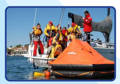
6. Board life raft and check that all components are satisfactory and prepare to separate from stricken vessel.
